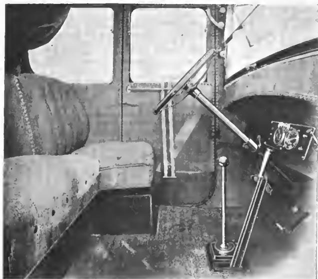
Inside view of Allen coupé. Note roominess for passengers in front seat. The driver's seat is located slightly in advance of the other, so that there will be ample space for manipulation of the control levers. The price is $1,075
